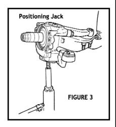
the jack only) **(FIG. 3).**Strike the top of the axle with a large hammer just behind the knuckle to seat the king-
