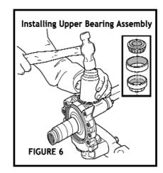
on kingpin to 200 ft. lbs. After tightening remove bottle jack from bottom of king pin. Rotate knuckle back and forth several times to make sure knuckle turns freely. If no binding occurs tighten kingpin to 600 ft. lbs.
