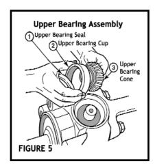
a suitable bearing driver to "TAP" the bearing assembly into the knuckle far enough down the kingpin threads to get the nut started on the kingpin (FIG. 6). Tighten nut
