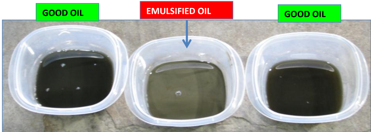
Figure 3: Oil with large amount of water has a light, milky appearance that is permanent.
