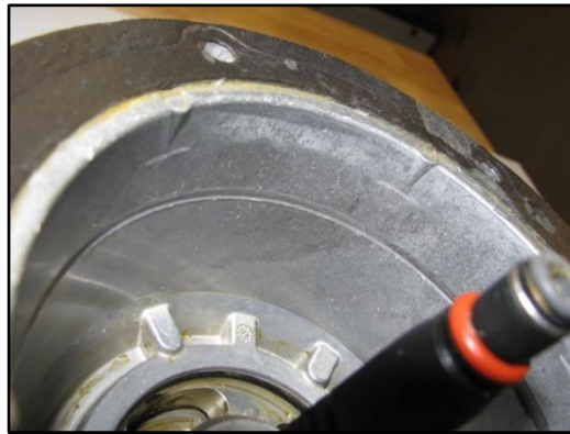
Interference occurs between the axle nut and hubcap, cutting into the hubcap wall
