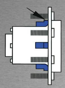
Locate one hub pilot pad at twelve o'clock position.
