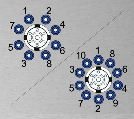
Complete procedure by tightening all the nuts in sequence shown to the recommended 450-500 ft.-lb. After installation, rotate wheels to be sure that the drum remains fully seated against the hub face.
