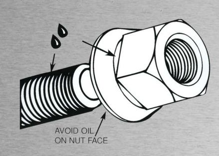
Apply two drops of oil on leading threads of studs and between nut body and flange. Avoid getting oil on face of nut, wheels, or brake drum.
