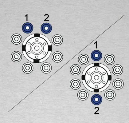
Finger tighten nuts on top two positions on an 8 hole wheel; top and bottom positions on a 10 hole wheel. Apply remaining nuts fingertight. Then snug all nuts to 50 ft.-lbs. following the sequence shown in step 6.
