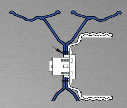
With wheels square to hub, mount inner and outer wheels as far back on the pilot pad as possible. Be sure both tire valve stems are accessible.
