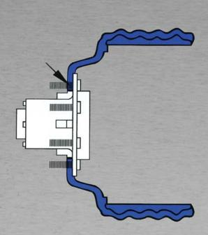
Before mounting wheels, be sure drum is properly positioned on raised step of pilot pad.
