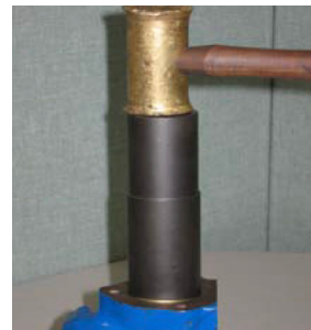
Use brass or dead-blow hammer to install
