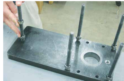
UPPER PLATE WITH FOUR 6 1/2" THREADED MOUNTING RODS AND ONE 6 1/2" LEVELING THREADED ROD WITH EXTRA NUT
